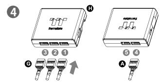
Connect the plug into the port in numerical order, start with plug one.
