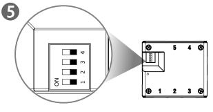
Set the DIP switch on the back side of the controller to assign the number of the controller
