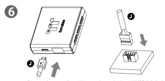
Connect the controller cable onto the motherboard (USB 2.0, 9 pin) and the controller.
